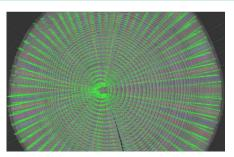
A path can run across a sample (core or disk radius) on a straight line. Hundreds of paths can be created with a single mouse click in predefined directions around the clicked position. Paths can aslo be created by clicking at their beginning and ending points.
