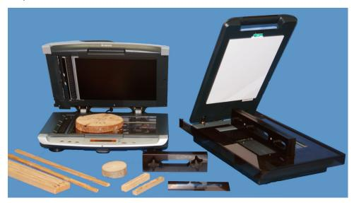
**WinDENDRO** analyses tree rings from wood disks, cores, X-Ray films and digital (filmless) X-Ray systems.
